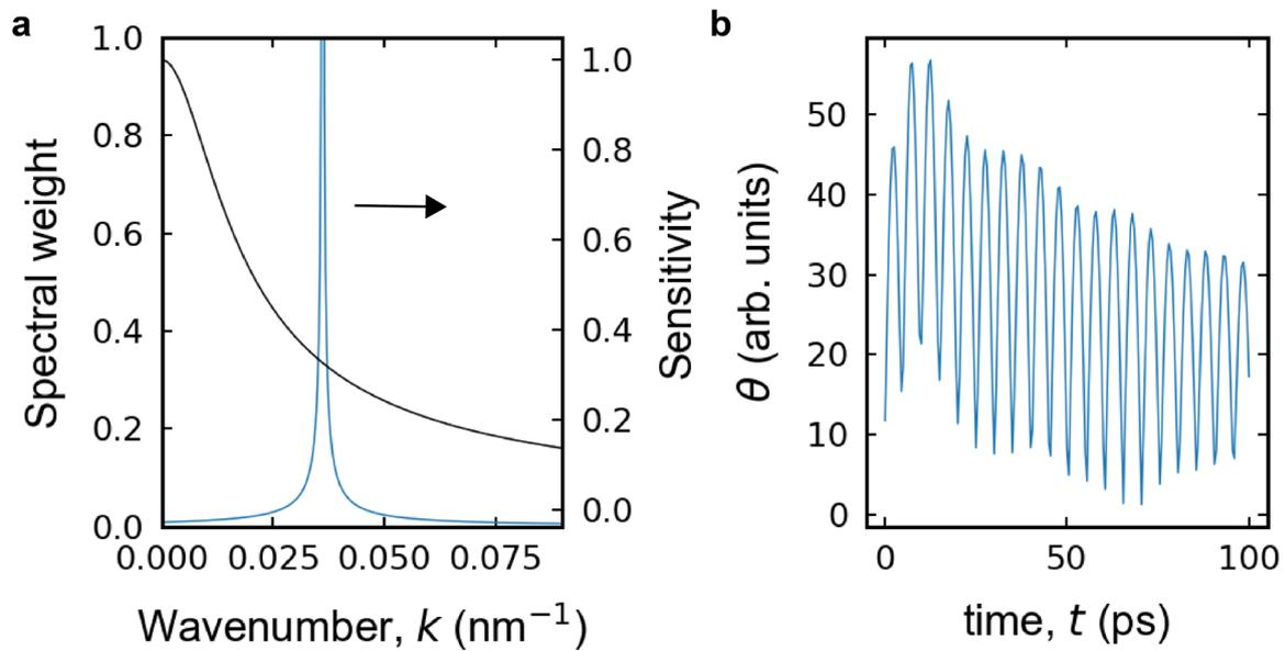
**Figure S2:** a) Wavepacket distribution (black line, left axis) and the sensitivity function as given by the first term of the integrand in Eq. S1.17 (blue line, right axis). b) The resulting time-resolved MOKE signal, given by the wavepacket distribution and the sensitivity function from panel a).
