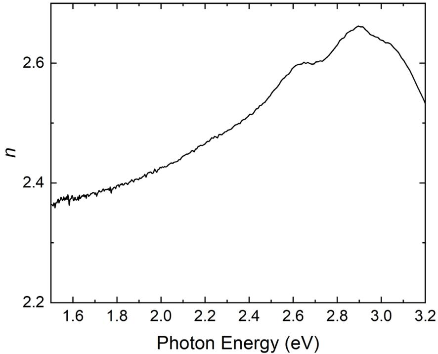
**Extended Data Figure 3: Real part of the refractive index as a function of the pump photon energy.** Real part  $n$  of the refractive index, as extracted using spectroscopic ellipsometry measurements.
