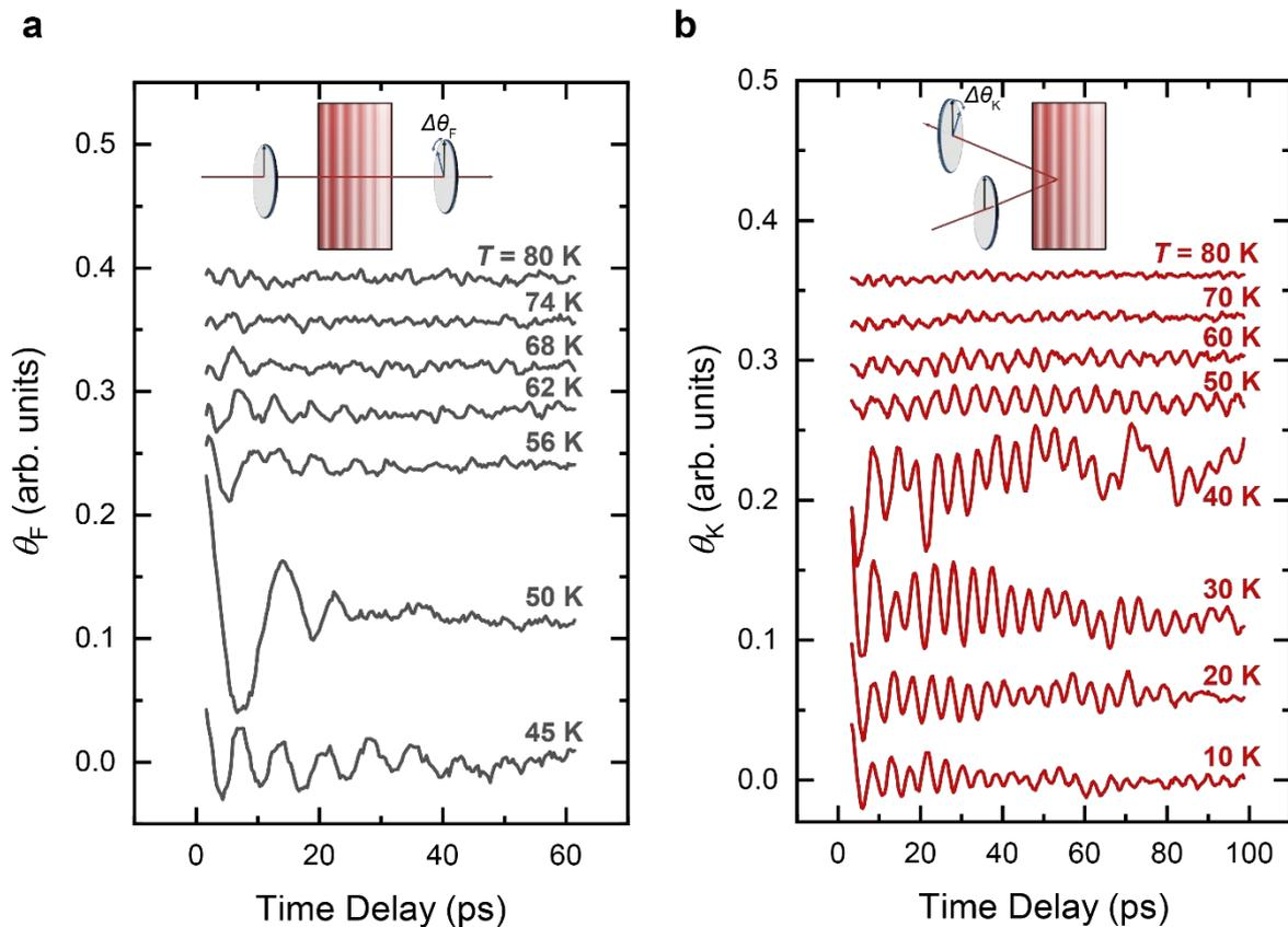
**Extended Data Figure 2: Magnon time traces at different temperatures.** a) Time resolved polarization rotation in the transmission (a) and reflection geometry (b) following excitation at  $h\nu = 3.1$  eV at different temperatures. The probe incidence angle is near-normal, with  $\lambda = 640$  nm and  $\lambda = 700$  nm for the measurements in panel a and b, respectively.
