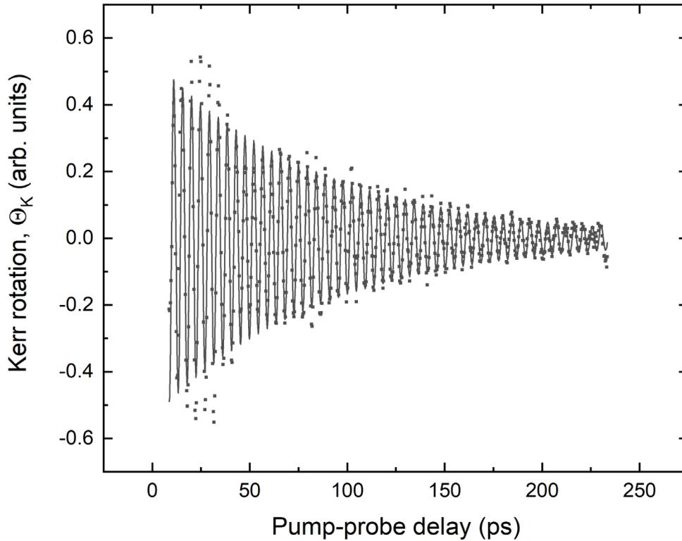
**Figure S4:** Time-resolved polarization rotation originating from a propagating magnon, as obtained in the reflection geometry. The solid line represents a best fit of a damped sine, giving a lifetime of  $\sim 85$  ps.
