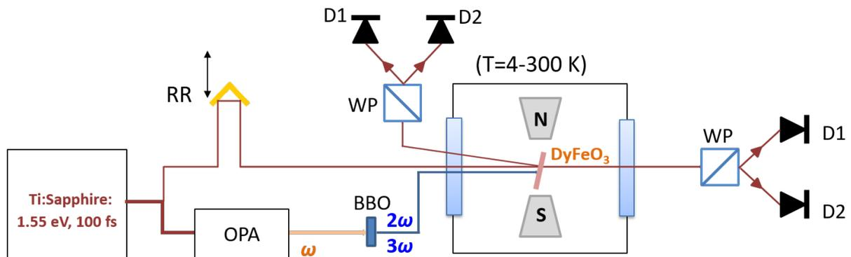
**Extended Data Figure 1: Experimental setup.** RR: gold retroreflector mounted on a motorized precision delay stage, OPA: optical parametric amplifier, BBO:  $\beta$ -barium borate crystal, WP: Wollaston Prism, D1, D2: pair of balanced silicon photodetectors.
